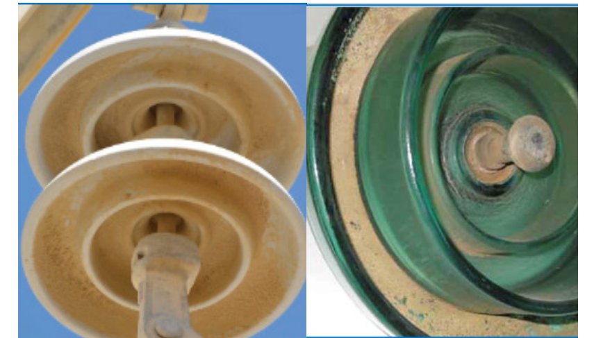
C&P insulators with pollution accumulation on underribs
