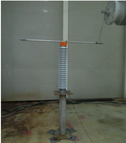
Figure 8 shows the set-up of the standard creepage RG insulator
