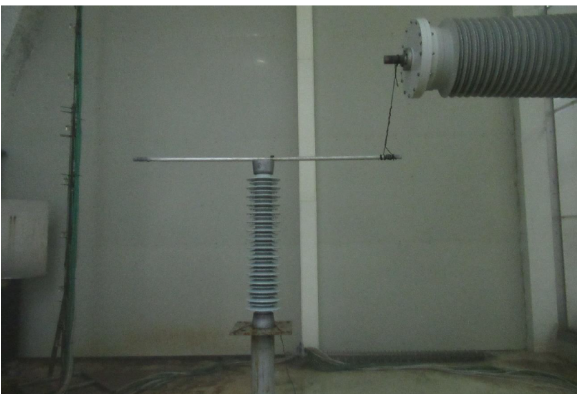
Figure 6 shows the high creepage insulator set-up
